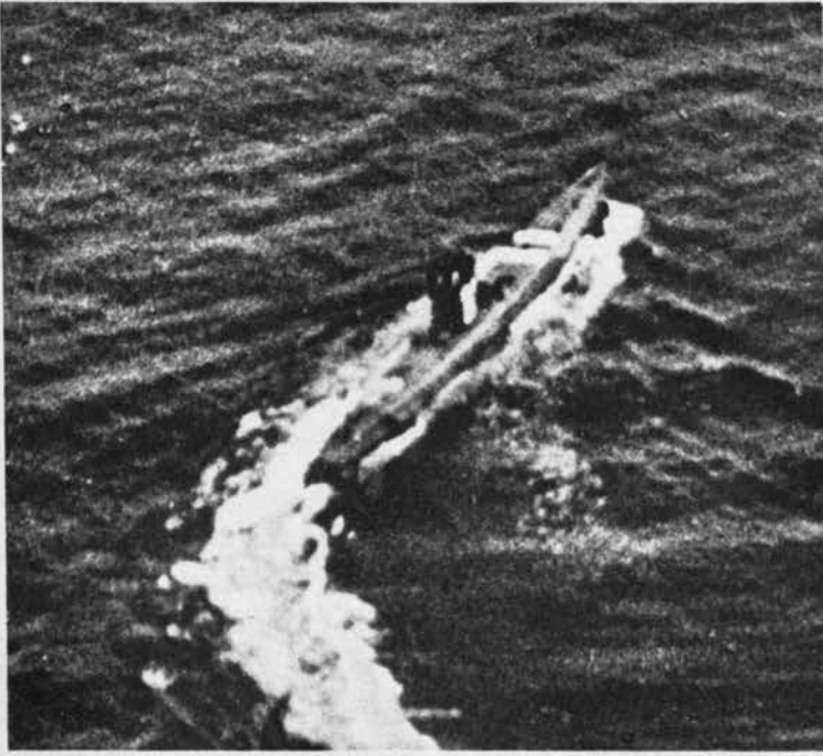
RO-100 CLASS COASTAL TYPE HAS TALL, BLOCKY TOWER SET AMIDSHIPS
